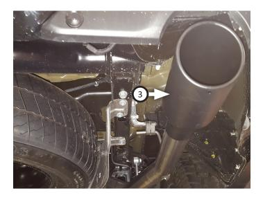
9. Place **tip (3)** onto left tailpipe. Tighten inlet to secure connection.
