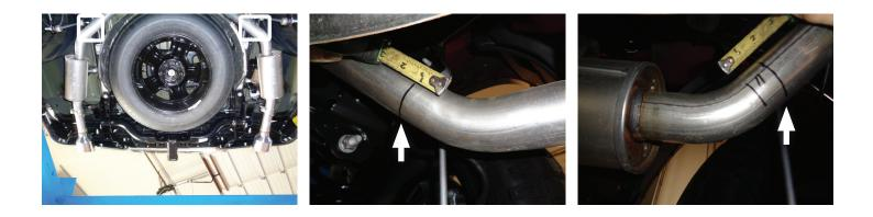
4. Cut driver and passenger side tailpipes off at marked lines and remove them from vehicle.
