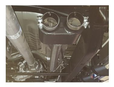
11. Fasten frame hanger (10) to vehicle frame (behind rear driver tire) with bolt (14), (x2) backing plates (11), flat washer (15), lock washer (16) and nut (17). Then fit rubber hanger (12) onto frame hanger.
