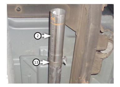
10. Place (x3) clamps (13) onto muffler (3) then connect it to inlet/extension pipe. Tighten front clamp just enough to allow for adjustment.
