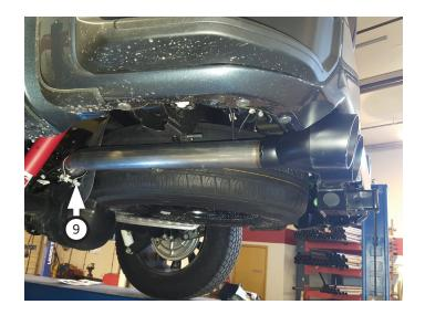
17. Place clamp (9) and isolator (removed step 8) onto right rear tailpipe (6) then connect it to right front tailpipe. Fasten isolator with bolt then tighten clamp enough to allow for adjustment.
