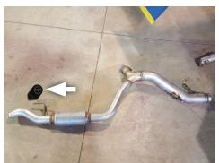
9. Disassemble inlet pipe wire hanger from isolater. Loosen factory clamp at catalytic converter and remove remaining muffler assembly from vehicle.
