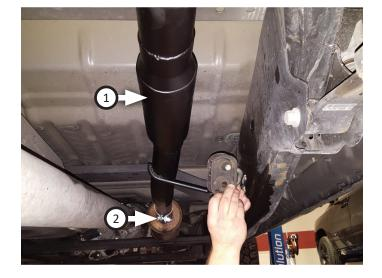
We recommend applying a one inch tack weld to all slipfit connections for a more secure installation. You may also apply high temperature paint over welded areas to prevent rust and premature corrosion.
