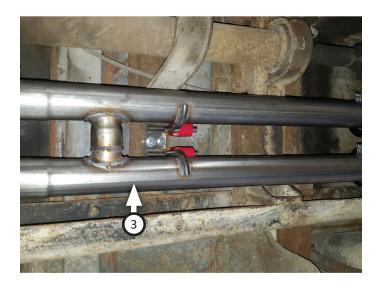
Place (x2 ea.) clamps (13) onto mufflers (4) then connect them to h-pipe assembly. Tighten clamps just enough to allow for later adjustment. Place (x2) clamps (13) onto end of mufflers.
