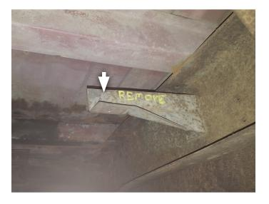
On crossmember above spare tire, make two marks inward from intersecting frame; driver side: 4½" inward, passenger side: 2½" inward. Use (x2) rear hangers (14) oriented as shown to drill (x4) <sup>5</sup>/<sub>16</sub>" mount holes.
