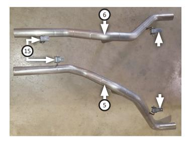
Route right tailpipe over axle and connect it to muffler. Fasten front and rear hangers to vehicle frame with (x3) **bolts (17)**, (x6) **flat washers (19)**, (x3) **lock washers (20)** and (x3) **nuts (18)**.
