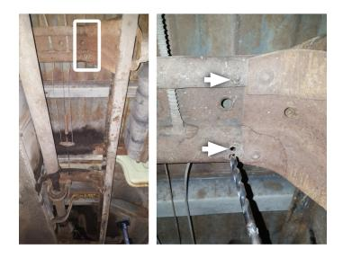
Mark line on front crossmember 2¼" outward from tank bracket as shown. Use front frame hanger (12) oriented as shown to drill (x2) <sup>5</sup>/<sub>6</sub>" mount holes.
