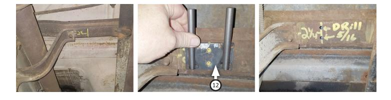
Fasten front frame hanger to crossmember with (x2) bolts (17), (x4) flat washers (19), (x2) lock washers (20) and (x2) nuts (18). Place (x2) rubber hangers (16) onto hangers as shown.
