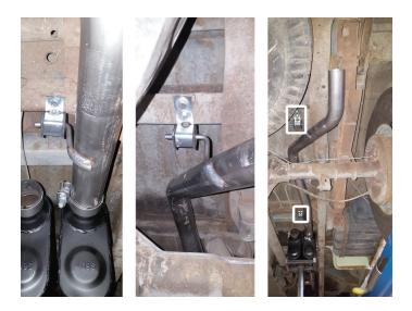
14. Route left tailpipe over axle and connect it to muffler. Fasten front and rear hangers to vehicle frame with (x3) **bolts (17)**, (x6) **flat washers (19)**, (x3) **lock washers (20)** and (x3) **nuts (18)**.
