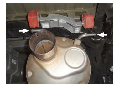
6. Remove nuts from factory pipe and catalytic converter flange. Remove muffler and factory pipe from vehicle.
