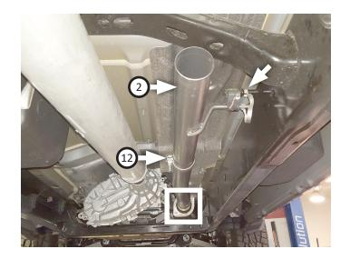
11. Place (x3) **clamps (12)** onto **muffler (3)** then connect it to extension pipe. Tighten front clamp just enough to allow for adjustment.
