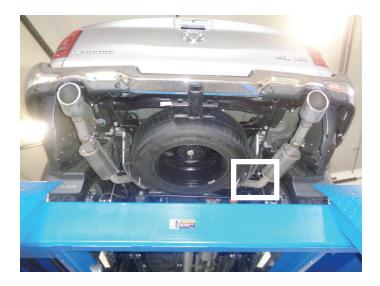
Remove factory tailpipe from vehicle by cutting it near muffler outlet and dismounting wire hangers from factory mounts. Remove and retain tailpipe isolators for later use.
