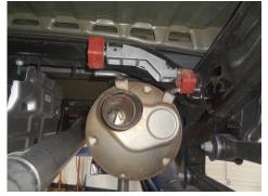
5. Remove factory muffler wire hangers (x3) from factory isolators and detach grounding wire.
