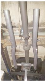
9. Place (x2 ea.) clamps (11) onto mufflers (4) then connect them to h-pipes and tighten clamps enough to allow for later adjustment.
