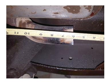
5. Mark forward cross member on both sides, inboard 2½" from intersecting frame edge.
