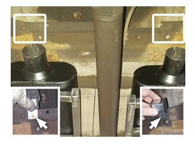
11. Set (x2) clamps (11) onto muffler outlets. Place (x2) rear hangers onto right (5) and left (6) tailpipes.
