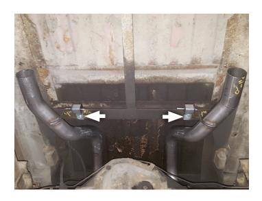
13. Secure (x2) front hangers (on tailpipes) to crossmember (step 10) with (x2) **bolts (15)**, (x4) **flat washers (17)**, (x2) **lock washers (18)** and (x2) **nuts (16)**.
