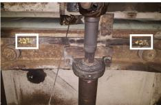
6. Use (x2) rear frame hangers (14) (oriented flanges out) to drill 5%6" mount holes then install hangers with (x2) bolts (15), (x4) flat washers (17), (x2) lock washers (18) and (x2) nuts (16).
