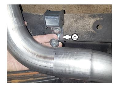
11. Place (x2) clamps (18) onto muffler (7) then connect it to muffler inlet pipe. Tighten front clamp just enough to allow for adjustment.
