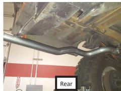
13. Place clamp (18) onto left (11) and right (10) exit turndown pipes then connect them to muffler exit. Tighten clamps just enough to allow for adjustment.
