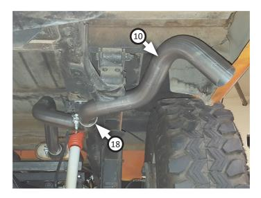
14. It will be necessary to adapt from your existing headers or manifold downpipes to the Flowmaster H-pipe assembly. Due to the many different variables in header/manifold down pipe locations, we have included right (1) and left (2) header adapters. Additional fabrication may be necessary to connect exhaust.
