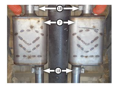
Route left (9) and right (8) muffler exit over axle and connect them to mufflers. Insert wire hangers into brackets then tighten clamps just enough to allow for adjustment.
