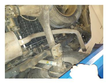
4. Support muffler and disassemble wire hangers from isolators. Remove and retain (x2) bolts and springs from flange then disconnect and remove muffler section from vehicle.
