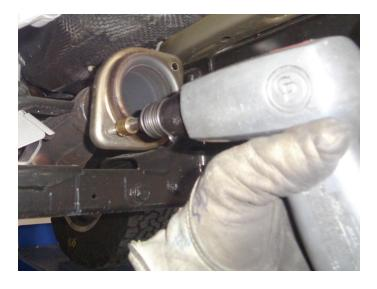
8. Remove nuts from stock and Flowmaster clamps, apply anti-seize compound to bolts and re-install nuts.
