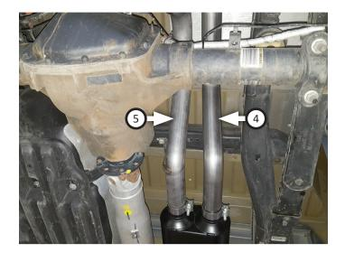
13. Place clamp (13) onto left rear tailpipe (6) then connect it to left front tailpipe. Insert wire hanger into rubber hanger then tighten clamp just enough to allow for later adjustment.
