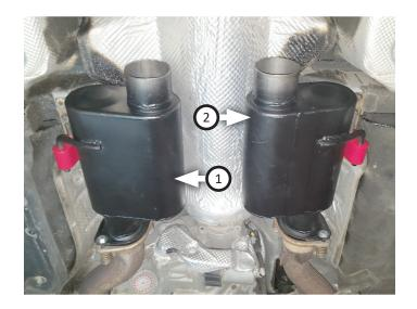
9. Place (x2) clamps (8) onto scavenger assembly (3) then connect it to resonators.
