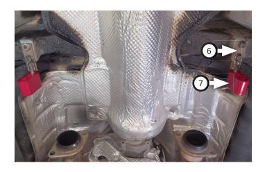
8. Connect left (1) and right (2) resonators onto inlets, inserting wire hangers into isolators. Secure flanges with (x2 ea.) bolts (9), flat washers (11), spacers (10) springs and nuts (removed step 4).
