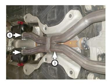
10. Place clamp (8) onto left muffler (5) then connect it to left side of scavenger assembly, fitting wire hanger into isolator. Tighten clamps just enough to hold parts.
