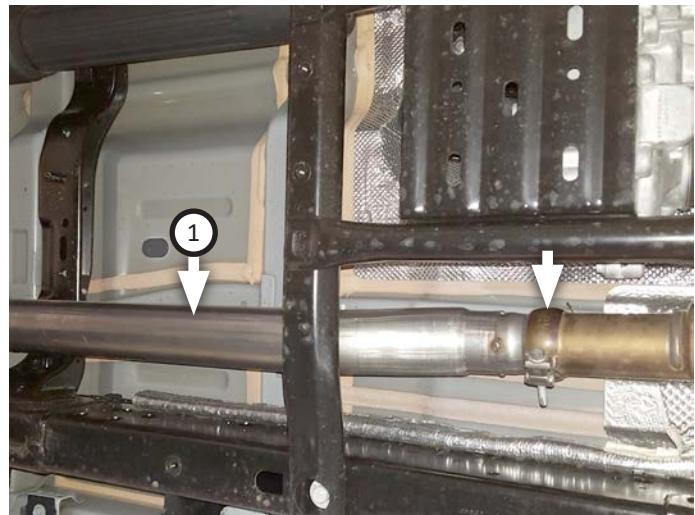
7. Place **clamp (3)** onto **muffler (2)** then connect it to inlet pipe. Tighten clamp just enough to allow for adjustment.
