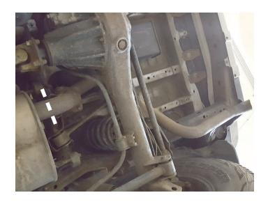
4. Support muffler and disassemble wire hangers from isolators. Remove and retain (x2 ea.) bolts and springs at both front flanged connections then remove muffler assembly.
