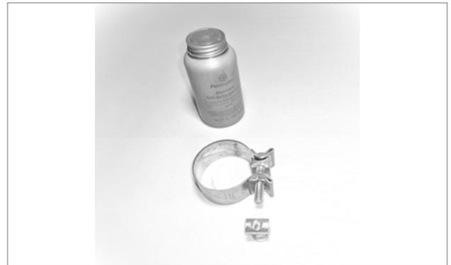
8. Prepare the clamp (4) by applying anti-seize compound to the bolt threads.
