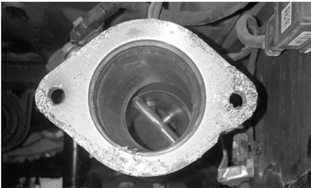
5. Remove the old gasket, and clean the flange of any remaining gasket material.
