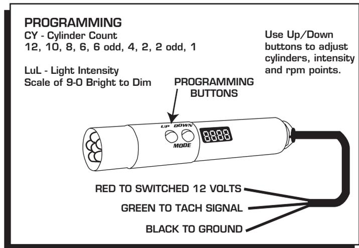
Figure 1 Digital Shift Light Wiring and Programming.
