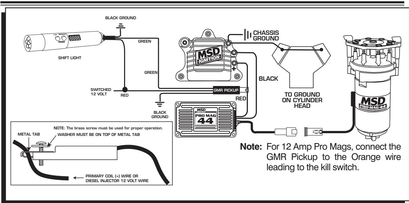
Figure 7 Wiring the Pro Mag 44 Electronic Points Box.
