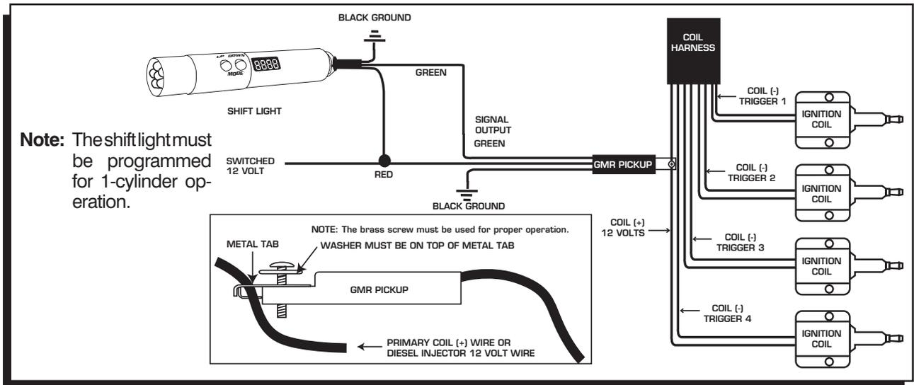
Figure 5 Installation on an Inductive Coil-Per-Cylinder Ignition System.
