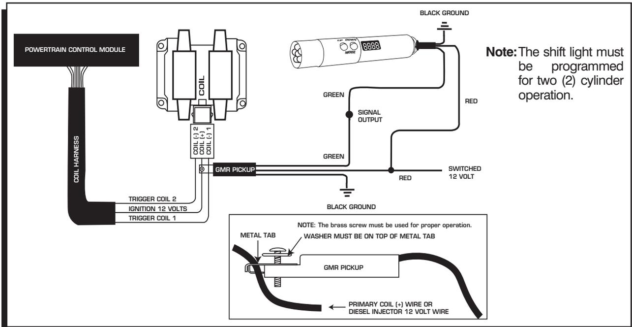
Figure 6 Installing to an Inductive Coil Pack.
