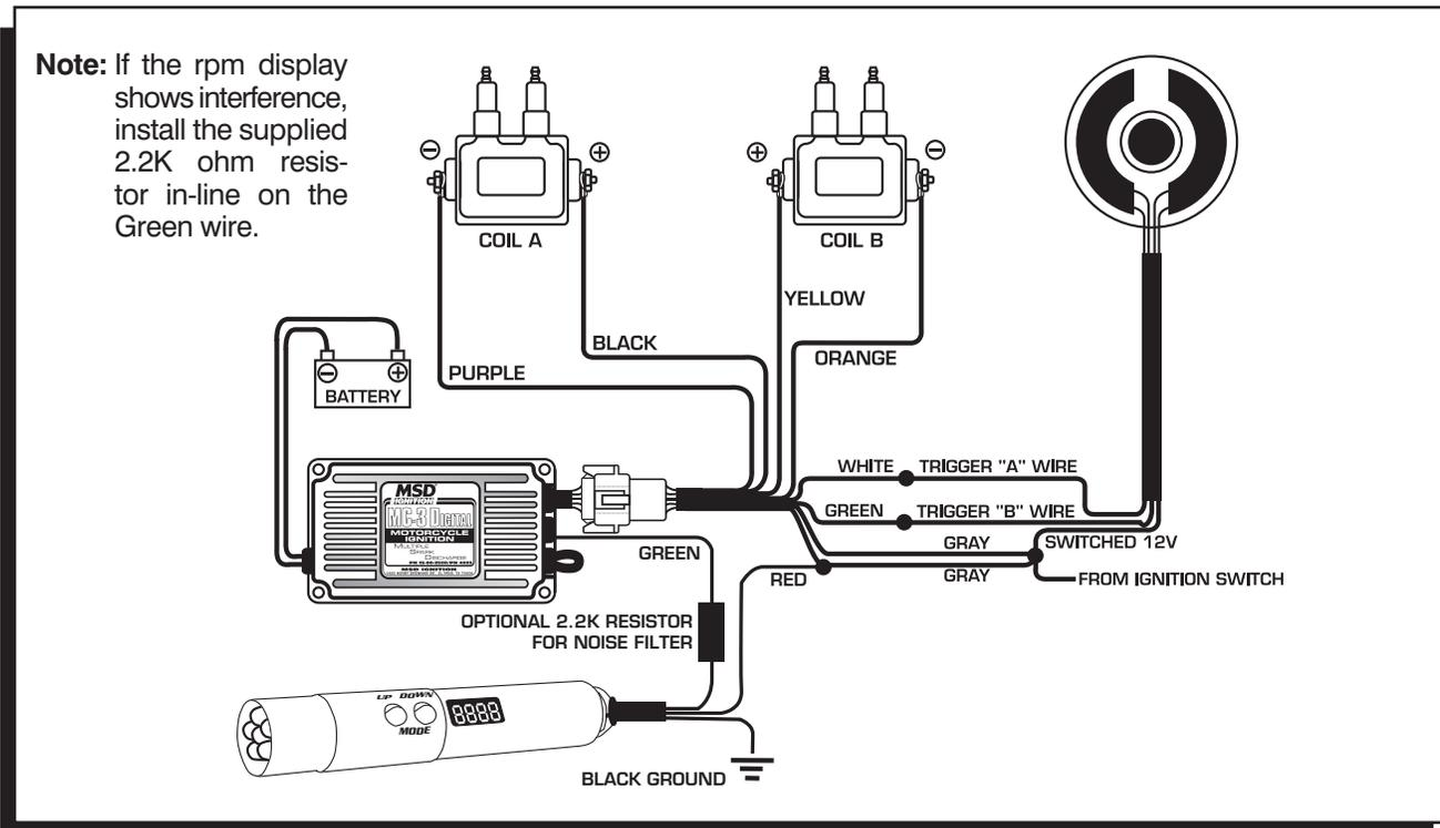
Figure 3 Installing with an MSD Motorcycle Ignition.
