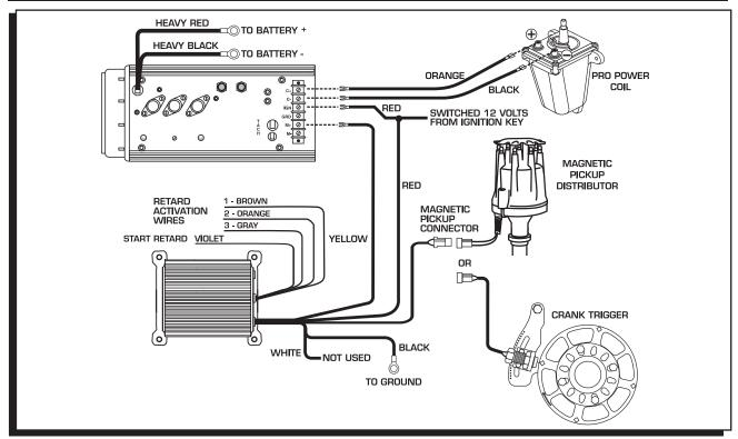
Figure 8 Wiring to an MSD 8 with a Mag Pickup.
