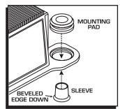
Figure 2 Installing the Vibration Mounts.
