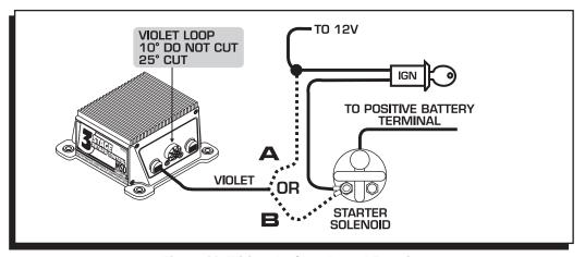
Figure 12 Wiring the Start Retard Function.
