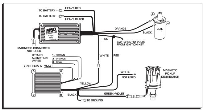
Figure 4 Wiring an MSD 6 Series Ignition with a Mag Pickup.
