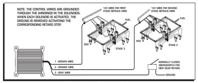
Figure 10 Wiring a Complete Retard System.
