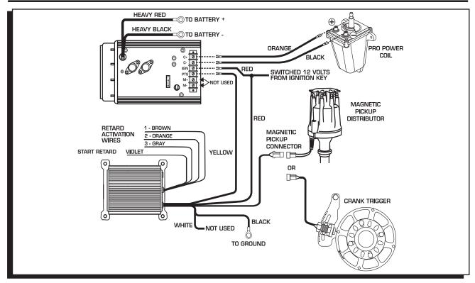
Figure 6 Wiring an MSD 7 Series Ignition with a Mag Pickup.
