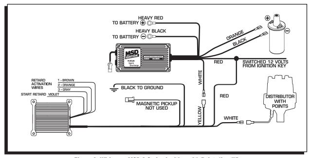
Figure 3 Wiring an MSD 6 Series Ignition with Points/Amplifier.
