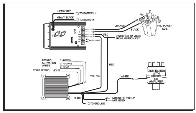
Figure 5 Wiring an MSD 7 Series Ignition with Points/Amplifier.
