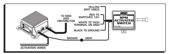
Figure 11 Activation with an RPM Activated Switch.
