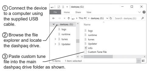
NOTE: The custom tune file must be placed in this exact location in order for the device to read and import it. Once the device recognizes it and imports it automatically, you will recieve verification on the screen stating that "Custom Tune for VIN.... has been loaded".
